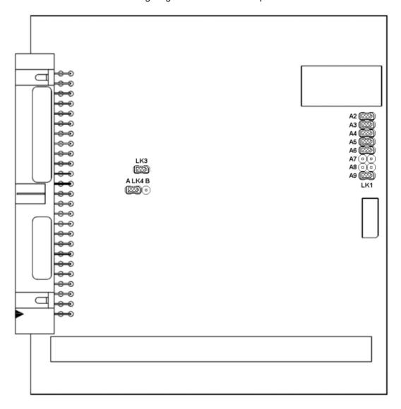
Use links LK3 and LK4 to select the analogue input channel configurations. For 16 channel single ended operation, insert LK3 and insert LK4 in position A. In this configuration, PDIFF should be used as the ground reference. For 8 channel differential operation, remove LK3 and insert LK4 in position B.
